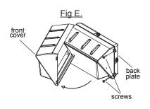
Drill the 4 (A) holes on the back plate needed to install on your J-box. Remove center knockout (C). Make sure power is off. Feed power supply wires thru the knockout hole (Fig. F).
