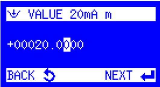
6. Input a 20 mA value. In this example, **20** will be entered. After entering a value, press the Enter key.
