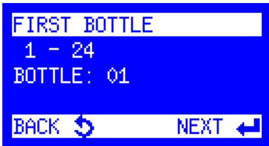
7. **First Bottle** is displayed if the ProSample has more than one bottle installed. Enter the bottle number in which the first sample should be placed. Press the Enter key.
