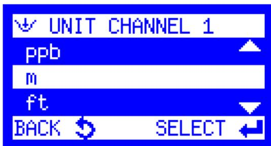
4. The **Unit** does not ultimately impact the measurement result, but a unit does need to be used. In this example, m will be used as the 'dummy' unit. After highlighting a unit, press the Enter key.
