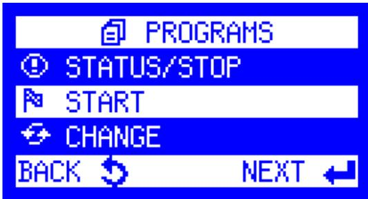
15. To run the program, highlight **Start** and press the Enter key.
