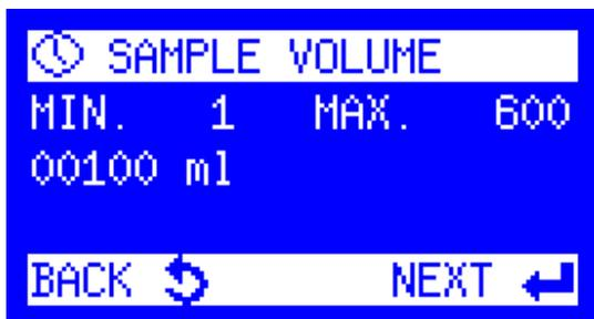
4. The **Sample Volume** is displayed. This is the amount of sample that will be collected at each Sampling Interval. The Sample Volume is determined by the user based on the application and sampling requirements. Press the Enter key to begin modifying the program.
