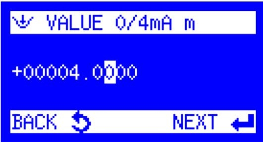
5. Input a 0/4 mA value. In this example, **4** will be entered. After entering a value, press the Enter key.
