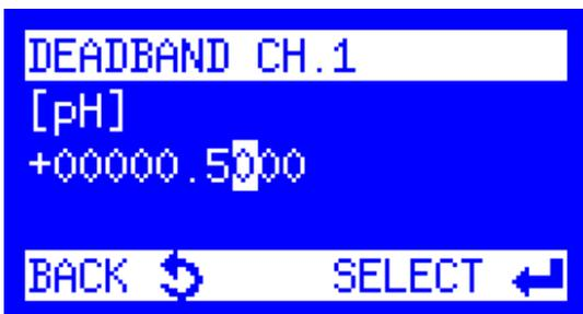
7. The ProSample will request a **Deadband** be entered. Deadband is important when using the Event method of sampling, but *Deadband is not relevant with the Continuous method (any value can be entered since ProSample will continue to run the program until completion).*
