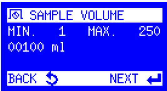
15. The **Sample Volume** is displayed. This is the amount of sample that will be collected at each Sampling Interval. The Sample Volume is determined by the user based on the application and sampling requirements. Press the Enter key to begin modifying the program.
