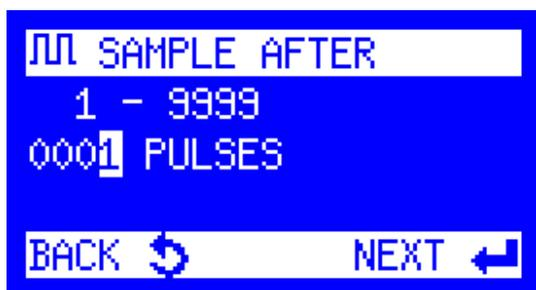
3. Enter 0001 for **Sample After**. The data logger will send a pulse to the ProSample when a sample needs to be taken.
