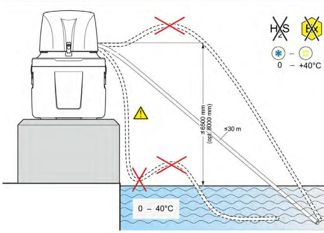
*Positioning of the ProSample unit and suction hose*
