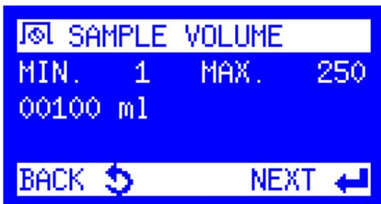
12. The **Sample Volume** is displayed. This is the amount of sample that will be collected at each Sampling Interval. The Sample Volume is determined by the user based on the application and sampling requirements. Press the Enter key to begin modifying the program.
