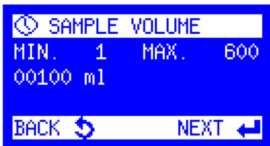
9. The **Sample Volume** is displayed. This is the amount of sample that will be collected at each Sampling Interval. The Sample Volume is determined by the user based on the application and sampling requirements. Press the Enter key to begin modifying the program.
