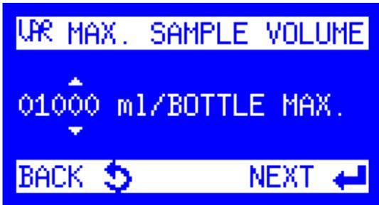
6. The **Var Sample Volume 20 mA** is displayed. This is the amount of solution that should be collected when the mA signal is 20 mA. Enter a value and press the Enter key.
