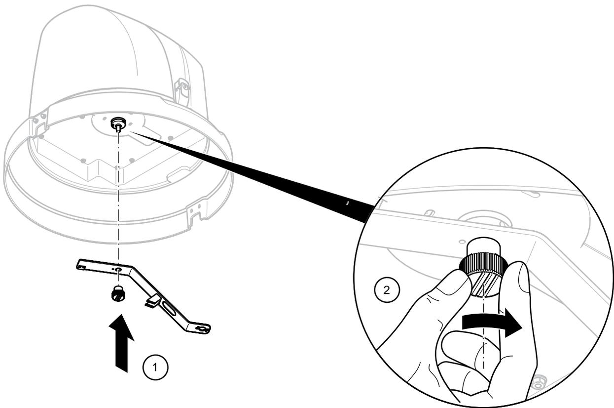
5. There is a plastic bracket on the bottom of the ProSample housing that keeps the distributor tube in place during sampling – place the distribution tube into this plastic bracket.
