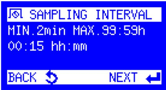
14. Enter a **Sampling Interval**. This determines how often a sample will be collected and is determined by the user based on the application and sampling requirements. Press the Enter key to begin modifying the program.
