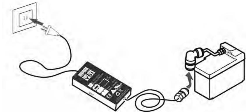
Connection of the ProSample battery to the battery charger
