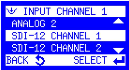
3. Highlight an **SDI-12 CHANNEL** to configure and press the Enter key.
