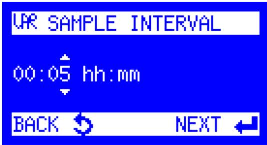
5. Enter a **Var Sample Interval**. This determines how often a sample will be collected and is determined by the user based on the application and sampling requirements.
