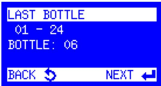
8. **Last Bottle** is displayed. Enter the bottle number in which the last sample should be placed. Press the Enter key.
