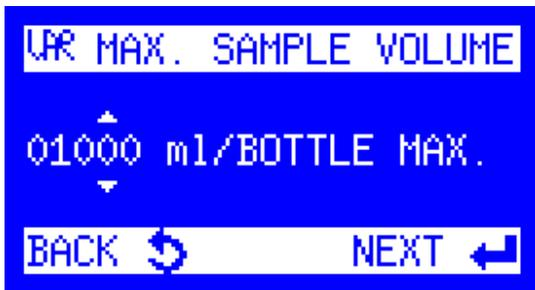
9. The **Var Max. Sample Volume** is displayed. Enter a value that is larger than the Var Sample Volume 20 mL (see step #6) but smaller than or equal to the maximum sample volume of the containers being used (e.g. 1000 mL when using 1000 mL bottles).
