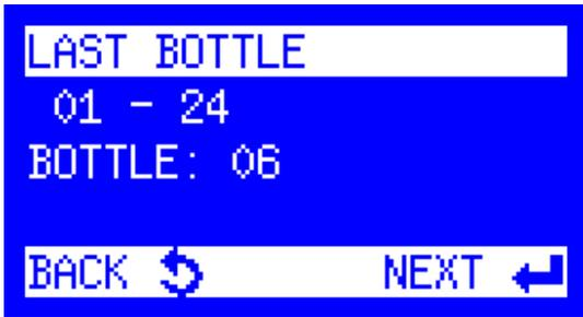
9. **Last Bottle** is displayed. Enter the bottle number in which the last sample should be placed. Press the Enter key.
