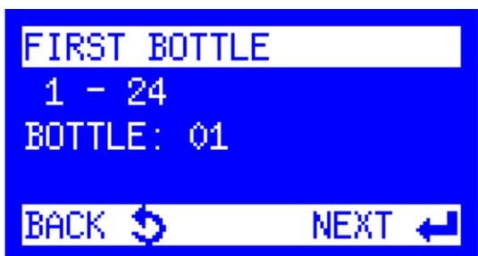
12. **First Bottle** is displayed if the ProSample has more than one bottle installed. Enter the bottle number in which the first sample should be placed. Press the Enter key.
