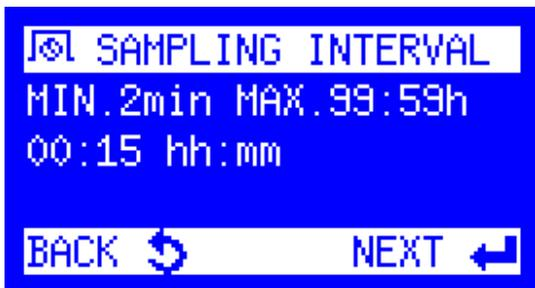
11. Enter a **Sampling Interval**. This determines how often a sample will be collected and is determined by the user based on the application and sampling requirements. Press the Enter key to begin modifying the program.
