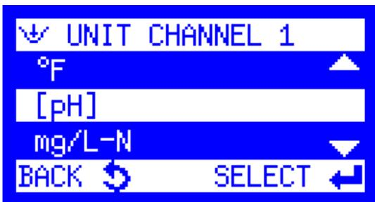
4. Select the appropriate **Unit** for the channel that is being configured and press the Enter key. In this example, pH is configured to be the Channel 1 unit, as pH is configured to be the channel 1 unit on the EXO3 sonde.
