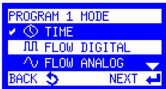
2. Highlight **Flow Digital** and press the Enter key.
