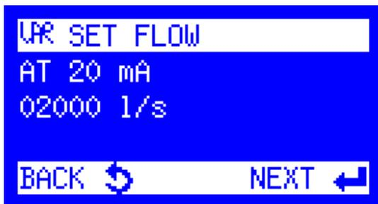
4. **Var Set Flow at 20 mA** is displayed. Although the value entered here ultimately does not impact the measurement result, it can be used to document the measurement value (e.g. flow) that corresponds to a mA signal of 20 mA. After entering a value, press the Enter key.
