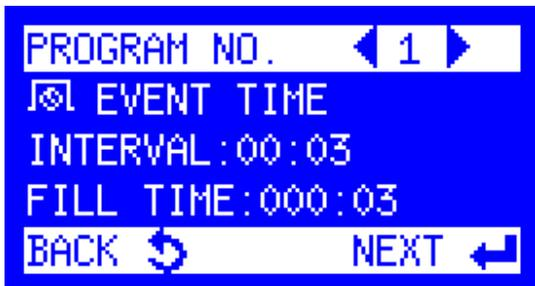
9. Press the Back key a few times to return to the Main Menu. Select **Programs** → **Change**. Choose the program you would like to modify by using the left and right arrow keys. A different channel must be configured for each SDI-12 parameter that will be used, but the trigger channel number and the program number do not need to be the same (e.g. the trigger/input channel could be #3, but this could be used for program #1). Press the Enter key to begin modifying the program.
