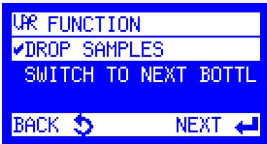
10. Highlight a **Var Function** and press the Enter key. This determines what will happen if there is more solution that will be placed in a bottle than the bottle can actually hold (see Var Max. Sample Volume). It is recommended to highlight **Drop Samples** and press the Enter key.
