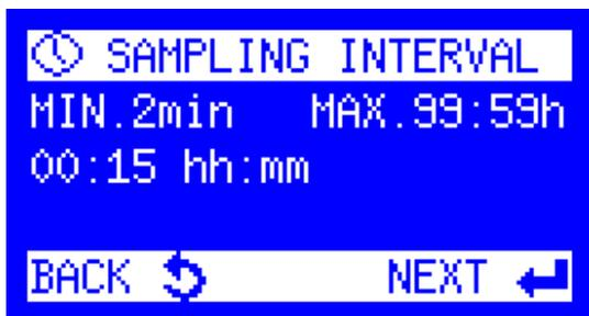
8. Enter a **Sampling Interval**. This determines how often a sample will be collected and is determined by the user based on the application and sampling requirements. Press the Enter key to begin modifying the program.
