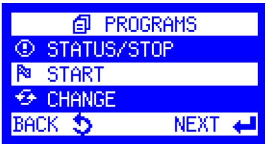
11. To run the program, highlight Start and press the Enter key.
