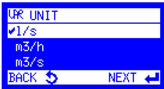
3. **Var Unit** is displayed. This ultimately does not impact the measurement result, but a unit does need to be used. In this example, l/s will be used as the 'dummy' unit. After highlighting a unit, press the Enter key.
