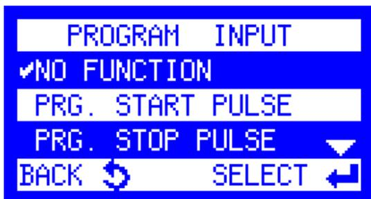
1. From the Main Menu, select **Setup** → **System Settings** → **Program Inputs** → **Program Input**.
