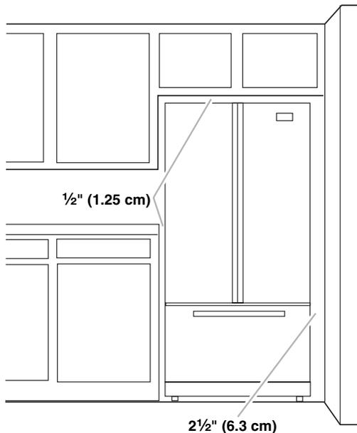
To ensure proper ventilation for your refrigerator, allow for 1/2" (1.25 cm) space on each side and at the top. Allow at least 1" (2.54 cm) between the back of the cabinet and the wall. If your refrigerator has an ice maker, allow extra space at the back for the water connections. When installing your refrigerator next to a fixed wall, leave 2 1/2" (6.3 cm) minimum on each side (some models require more) to allow for the door to swing open.
