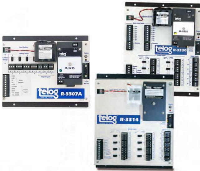
The R-33xx recorders become your eyes and ears in the field. The recorders accept analog and/or event inputs with a sample rate of 1 per sec up to 1 per 8 hours, storing up to 300,000 interval computations in memory. R-33xx units record output from a variety of sensors such as pressure, level, flow, pH, temperature and humidity. Combine the R-33xx recorders with a power source and communication option to easily administer a network of hundreds of remote recorders.
