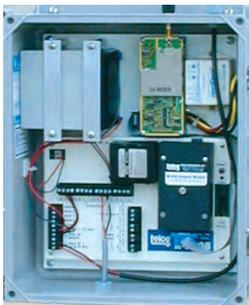
R-33xx recorders may be packaged with power source and communication option in a NEMA 4X enclosure.
