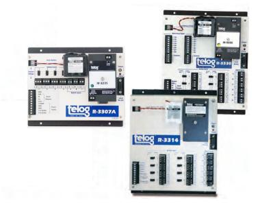
The R-33xx recorders become your eyes and ears in the field. The recorders accept analog and/or event inputs with a sample rate of 1 per sec up to 1 per 8 hours, storing up to 300,000 interval computations in memory. R-33xx units record output from a variety of sensors such as pressure, level, flow, pH, temperature and humidity. Combine the R-33xx recorders with a power source and communication option to easily administer a network of hundreds of remote recorders.
