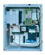
R-33xx recorders may be packaged with power source and communication option in a NEMA 4X encosure.
