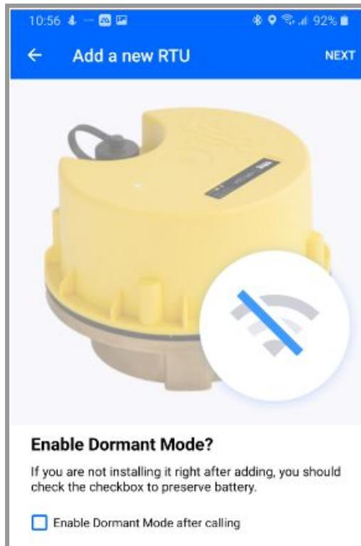
11. Tap on **Next**. The **RTU Added!** screen is displayed with a **Verifying communication** message and a progress status bar. The device is calling to connect to the app, performing a Tamper via Bluetooth, and registering the device to add to the list of RTUs.
