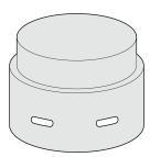
2. Press the **security cover** down firmly while inserting the narrow arm of a **security hasp** through a slot in the security cover from one direction and the narrow arm of the other security hasp from the other direction, so they overlap.
