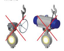
Fig. 2 Lifting the valve
