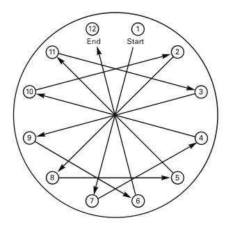
Fig. 8 Tightening sequence for 12 bolts
