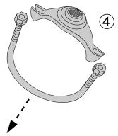
**Step 5** • Position the saddle body on the pipe such that the outlet is in the correct location.
