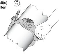
Step 7 • Tighten all nuts evenly in 20 ft-lbs. increments. Use a wrench with at least a 12 inch handle.
