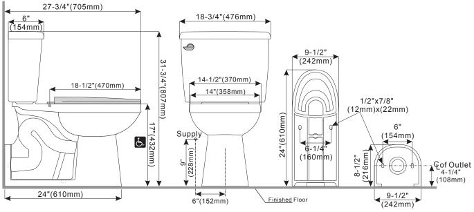
Note: All dimensions and specifications are nominal and may vary: Dimensions of 8" and greater have a tolerances of +3%. Dimensions less than 8" have a tolerances of +5%
