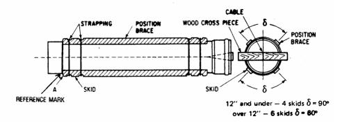
ensure the pipe is not "over-belled" or inserted beyond the maximum insert reference mark, the skids or casing spacers must be aligned with the
