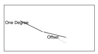
of curvature, assumes the spigot is not inserted beyond the insert reference mark. Inserting the spigot beyond the insert reference mark reduces allowable joint offset.
