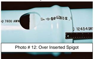
mark falls well short of the lip of the bell, the pipe needs to be pushed a little further until the mark is aligned. Here the cutaway shows that the joint has no flexibility, and cannot expand.
