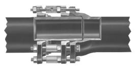
The AMERICAN MJ Coupled Joint is furnished in sizes 4"-48" and is an adaptation of the standard Mechanical Joint to provide joint restraint against thrust due to internal pressure.
