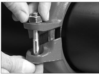
**6. INSTALL REMAINING BOLT/NUT:** Install the remaining bolt and thread the nut finger-tight onto the bolt. **NOTE:** Verify that the oval neck of each bolt seats properly in the bolt hole.
