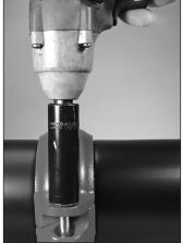
**5. TIGHTEN NUTS:** Tighten nuts evenly by alternating sides until metal-to-metal contact occurs at the angled bolt pads. Verify that the oval neck of each bolt seats properly in the bolt hole and that housings' keys engage the grooves completely on both mating components. Equal and positive or neutral offsets shall be present at the bolt pads.
