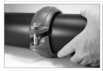
**4. ASSEMBLE JOINT:** Assemble the joint by inserting the grooved end of a mating component into each opening of the coupling. The ends of the grooved mating components shall be inserted into the coupling until contact with the center leg of the gasket occurs. A visual check is required to verify that the coupling keys align with the grooves in the mating components. **NOTE:** The coupling may be rotated to verify that the gasket is seated properly.
