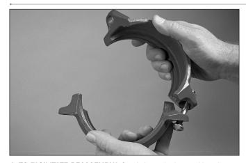
**4. TO FACILITATE REASSEMBLY:** One bolt can be inserted into the housings with the nut threaded loosely onto the bolt to allow for the "swing-over" feature, as shown above. **NOTE:** The nut should be backed off no further than flush with the end of the bolt.
