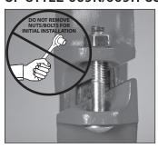
1. DO NOT DISASSEMBLE THE COUPLING: Style 009N/009H FireLock EZ™ Installation-Ready™ Rigid Couplings are designed so that the installer does not need to remove the bolts and nuts for installation. This design facilitates installation by allowing the installer to directly insert the grooved end of mating components into the coupling.
