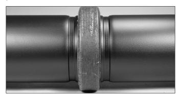
**5. JOIN PIPE/MATING COMPONENTS:** Align the two grooved ends of the pipe/mating components. Insert the other pipe/mating component end into the gasket until it contacts the center leg of the gasket. **NOTE:** Make sure no portion of the gasket extends into the groove of either pipe/mating component.
