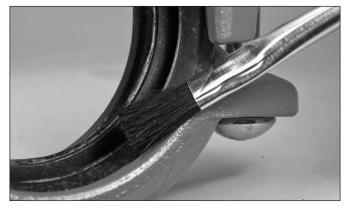
4. LUBRICATE GASKET: Apply a thin coat of Victaulic Lubricant or silicone lubricant only to the sealing lips of the gasket interior. NOTE: The gasket exterior is supplied with a factory-applied lubricant, so it is not necessary to remove the gasket from the housings to apply additional lubricant to the exterior surface.
