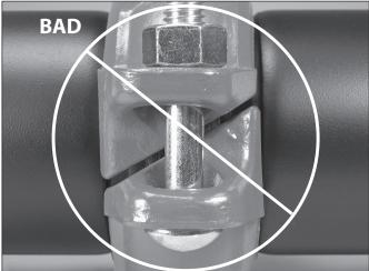
7. Visually inspect the bolt pads at each joint to ensure metal-to-metal contact is achieved
