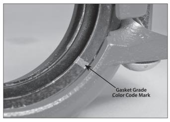
3. CHECK GASKET: Check the gasket to make sure it is suitable for the intended service. The color code identifies the gasket grade. Refer to Victaulic publication 05.01 in the G-100 General Catalog or the I-100 Field Installation Handbook for the color code chart.
