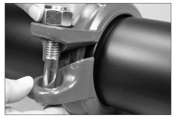
**8. INSTALL REMAINING BOLT/NUT:** Install the remaining bolt, and thread the nut finger-tight onto the bolt. **NOTE:** Make sure the oval neck of each bolt seats properly in the bolt hole.
