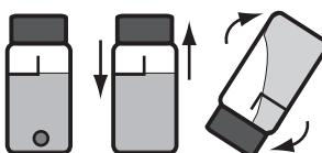
8. Immediately insert tube into chamber. Close lid. Select **Scan Sample**. Record result as Free Chlorine.
