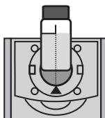
7. Remove tube from colorimeter. Add one DPD #1 IG Tablet [6903A]. Cap tube and shake for 10 seconds. Invert slowly 5 times. Solution will turn pink if free chlorine is present.
