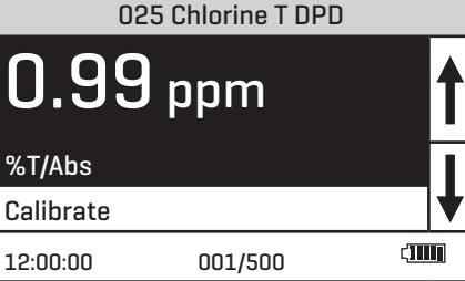
9. Press to select **Calibrate**. A reverse font [light background with dark characters] will appear to indicate that the reading can be adjusted.
