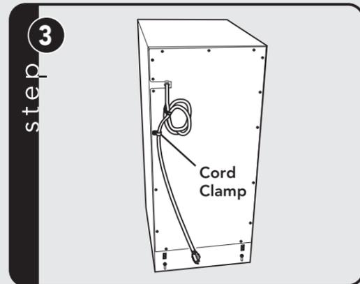
Use the cord clamp to prevent excess power cord from being pinched beneath the cabinet during installation or service.
