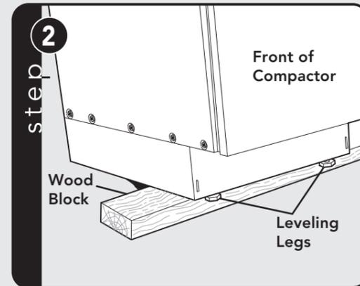
Tip the front of compactor up and onto a wood block. Turn the leveling legs in or out to the desired position. Remove the wood block.
