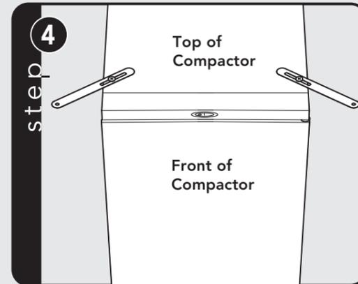
Fasten the slotted end of the straps to the compactor using the holes in the top of the compactor cabinet as shown.
