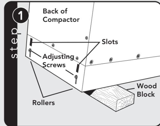
Tip the back of compactor up and onto a wood block. Loosen the adjusting screws only far enough to move the rollers to a higher or lower slot. Retighten the adjusting screws and remove the wood block.
