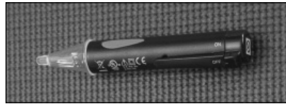
Figure 24 - Use a non-contact circuit tester to check for electrical power.
