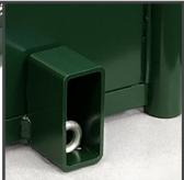
Lock Shield Brackets rest flush on the concrete to protect the forged eyebolts and padlocks against bolt cutters.
