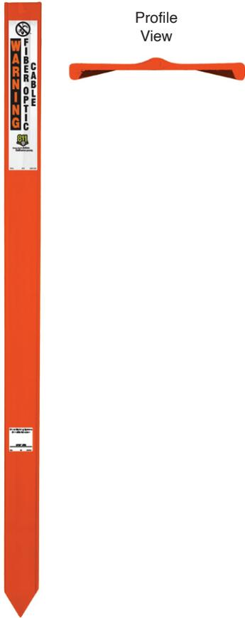
Rhino's 3-Rail fiberglass composite post uses the industry standard profile. It's our most drivable fiberglass marker and can be installed in almost any soil condition. The design allows for easy stacking and storing and has the durability to withstand repeated impacts when hit from the front or back.
