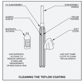
It is recommended that the UV lamp be replaced every two years to insure proper disinfection of the treatment system effluent. The green light on the side of the control enclosure will no longer illuminate when the lamp needs replaced. To replace the lamp:
