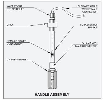
has become disconnected, it must be reconnected at this time. To do so, remove the gasketed cover from the control enclosure. Connect the lead labeled "ONE" on the UV power cable to the terminal block marked "1". Connect the lead labeled "TWO" to the terminal block marked "2". Connect the lead labeled "THREE" to the terminal block marked "3". Connect the yellow/green lead to the terminal marked "Y/G".
