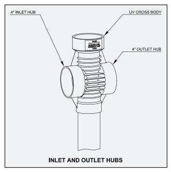
4. Solvent weld the effluent line of the upstream treatment system to the 4" inlet hub of the Model AT 1500. Next, solvent weld the 4" outlet hub to the final effluent line. Cover the open top of the disinfection chamber and backfill up to the bottom of the plumbing.
