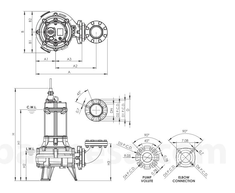
C.W.L.: Continuous Running Water Level L.W.L.: Lowest Running Water Level (Most effective motor heat dissipation when fully submerged)
