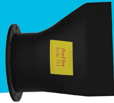
The **Proco Style 711 ProFlex™** check valves are engineered for installation on pre-existing pipe lines such as manholes, outfalls, vaults, where the outfall invert of the pipe is close to the floor of the manhole or outfall. When a new installation is being designed, the 711 valves can be engineered into the pipe layout with little concern for outfall clearance due to its “low slope” design.
