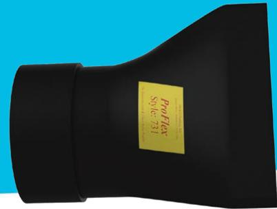
The **Proco Style 731 ProFlex™** check valves are engineered for installation on pre-existing pipe lines such as manholes, outfalls, vaults, where the outfall invert of the pipe is close to the floor of the manhole or outfall. When a new installation is being designed, the 731 valves can be engineered into the pipe layout with little concern for outfall clearance due to its “low slope” design.
