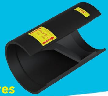
The **ProFlex™ 790** Low Headloss In-line Rubber Duckbill Check Valve design allows for a passive flow and allows the valve to be installed without having to do any modifications to existing structures or costly pre-install planning. The unique fold away design of the inner sleeve also allows for a near full port flow, allowing for quick drainage.
