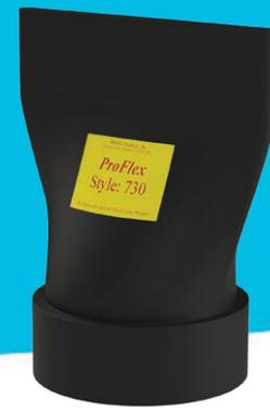
The **ProFlex™ 730** Slip-on Rubber Duckbill Check Valve is designed to slip directly over an existing pipe, and is supplied with heavy duty stainless steel clamp(s) to secure it in place. Sizes 1" - 10" utilize T-Bolt clamps and sizes above 10" utilize Bolt-On Clamps for securing.
