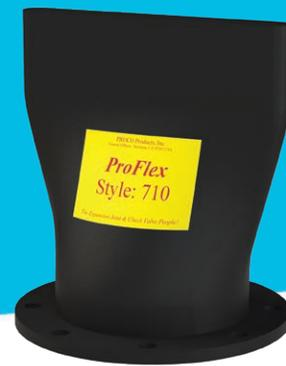
The **ProFlex™ 710** is a full port, concentric design Rubber Duckbill Check Valve. The ProFlex™ 710 Rubber Duckbill Check Valves can be supplied with many different flange drilling configurations, including square or rectangular flanges to suit problematic sluice gate or flap gate replacements.
