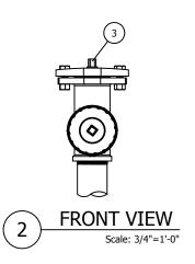
HYDRANT SHALL BE \_\_\_\_ ' BURY, WITH (2" MJ SIDE, 2" FIP SIDE, OR 2" FIP VERTICAL) INLET AND (ANY SIZE UP TO 2-1/2" NST) NOZZLE OUTLET.
