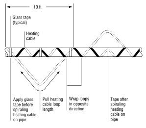
Figure 1. Spiraled heat tracing
