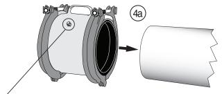
Connector for cathodic protection.
