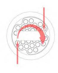
**EDGE ENGAGEMENT: 80 FT-LBS** TOOL ENGAGES VALVE KNOB EDGE MINIMIZING PINS ENGAGED.
