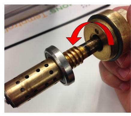
4) Take the new Spindle (TA-10) and insert into the cap assembly (T-12A). Thread the new spindle (TA-10) all the way into the cap clockwise until it rests flat against the spindle.
