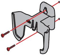
Mount the sensor vertically on an exterior wall, at least 6 inches below any overhang. Choose a location protected from direct sunlight.
