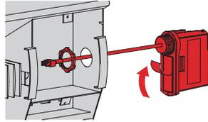
**2** Remove the locknut from the antenna and peel off the adhesive backing. Feed the antenna cable through the knockout and install the antenna vertically as shown. Put the locknut on and tighten.
