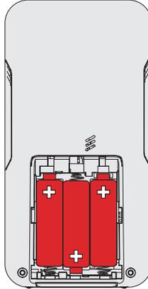
Install 3 AA alkaline batteries
