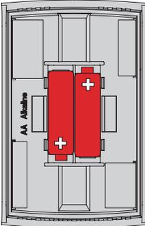
Install 2 AA alkaline batteries
