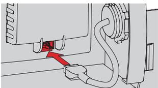
**5** Insert the antenna plug into the relay receptacle until you hear a click.
