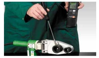
Important: If the pipe or the air around it is below 40 °F (5 °C), heating times are increased by 50%. Remember to take greater care with the pipe as it can become brittle in cold temperatures. Using power cutters on cold pipe can cause cracking and is not recommended. Use standard ratchet or wheel cutters instead. Never preheat the pipe beyond 100 °F (38 °C).
