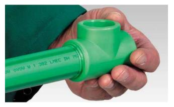
10. After the cooling period, the fused joint is ready for use. As the connection cools, the PP-R from the pipe bonds perfectly to the fitting, turning them into one piece. Within minutes, the connection is ready for full system pressure.
