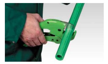
Always ensure that cutters are sharp. Cutting pipes with dull or damaged ratchet cutters can cause the pipe to crack.
