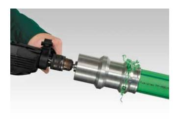
5. Clean the pipe again thoroughly, removing any burrs and smoothing the surface of the pipe.
