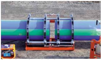
Open the clamps and remove heating element.
