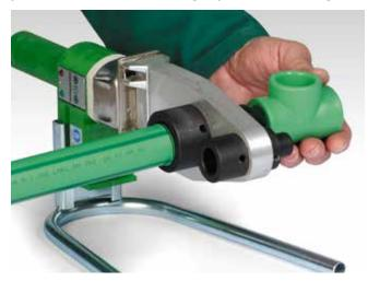
Warning: Welding heads and heating plate are extremely hot. Always use protective hand and arm coverings to reduce the risk of serious burns.
