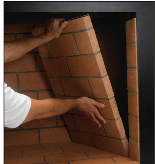
Pre-engineered firebrick wall system features steel reinforced, factory-built and grouted masonry walls that easily slip into place and securely fasten to the steel fireplace chassis.
