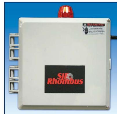
This panel provides a reliable means of controlling one single phase pump in water and sewage installations. Two control switches activate a magnetic motor contractor to turn the pump on and off. If an alarm condition occurs, an additional alarm switch activates the audio/visual alarm. **Approved for Halifax, Edgecombe, Warren, Wilson, Cleveland and Brunswick\* counties.**
