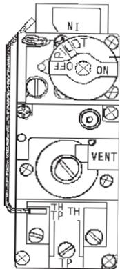
NOTE: Knob can not be turned from "PILOT" to "OFF" unless knob is pushed in slightly. Do not force.
