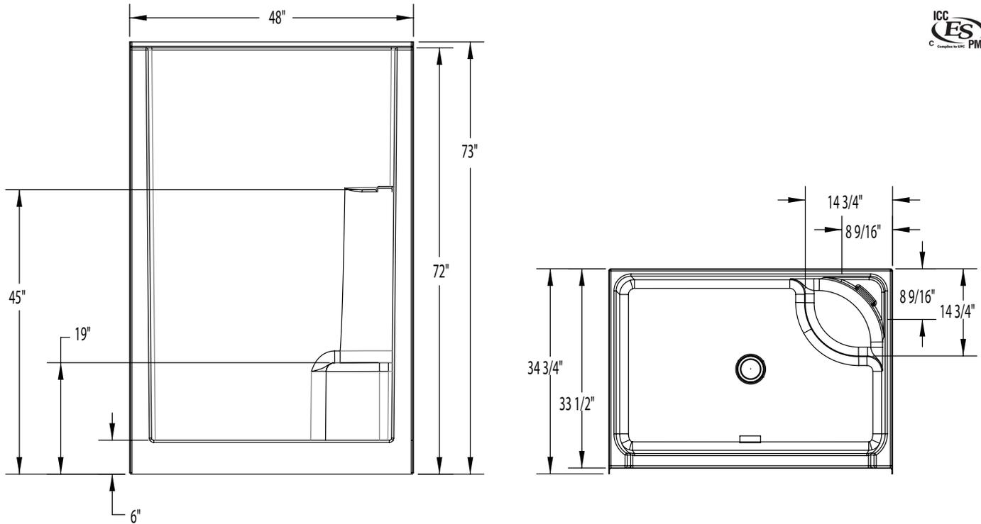
**FEATURES** lbs      Dimensional Tolerance  $\pm \frac{3}{8}$ ". Dimensions needed for site preparation should be measured from the unit. Aquatic assumes no responsibility for preparatory work.
