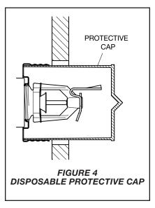
**Step 6.** After the wall has been completed with the nominal 2-1/2 inch (63,5 mm) diameter mounting hole and in preparation for installing the Cover Plate Assembly, remove and discard the Protective Cap and the Sprinkler Strap. If the Sprinkler has been damaged in any way including accidental over spray from finishing the wall, replace the entire Sprinkler/Support Cup Assembly.
