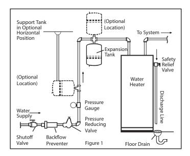
NOTE: If vertical installation is impractical, PFXT tank may be installed in a horizontal position as long as the tank weight is fully supported independent of the piping. The support can be in the form of strapping or a support platform. ABSENCE OF AN INDEPENDENT TANK SUPPORT WILL VOID THE WARRANTY.
