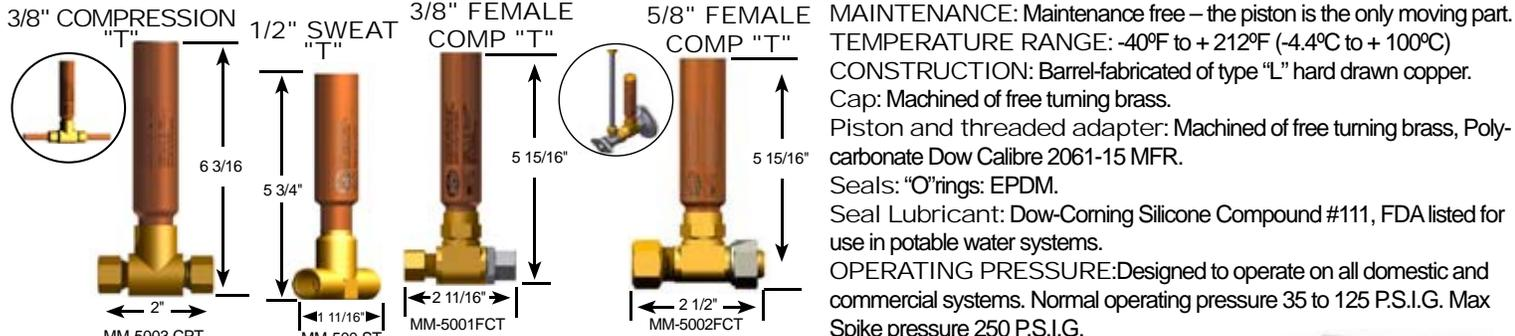
**MAINTENANCE:** Maintenance free – the piston is the only moving part.
