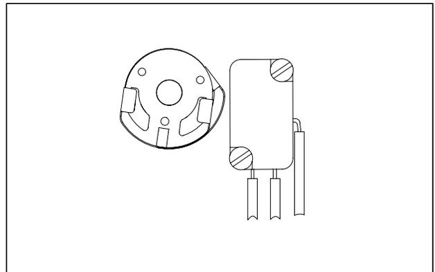
Fig. 9 Cams Set for Normally Closed Function
