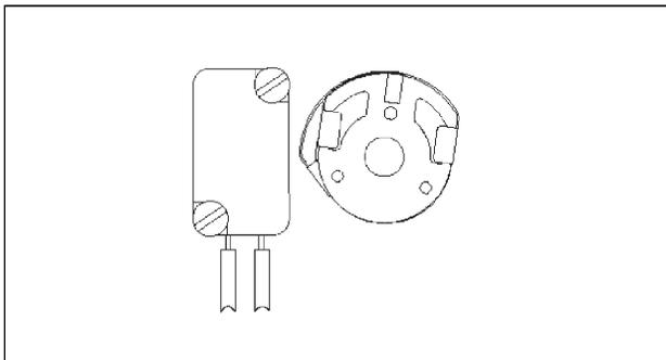
Fig. 13 Cams set for Normally Closed function
