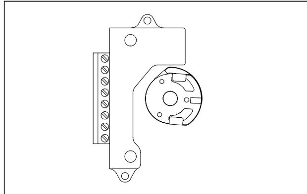
Fig. 5 Cams set for Normally Closed function
