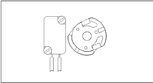
Fig. 12 Cams set for Normally Open function
