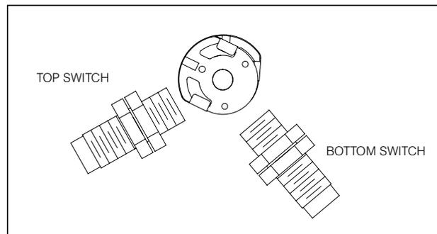
Fig. 11 Cams Set for Clockwise Rotation
