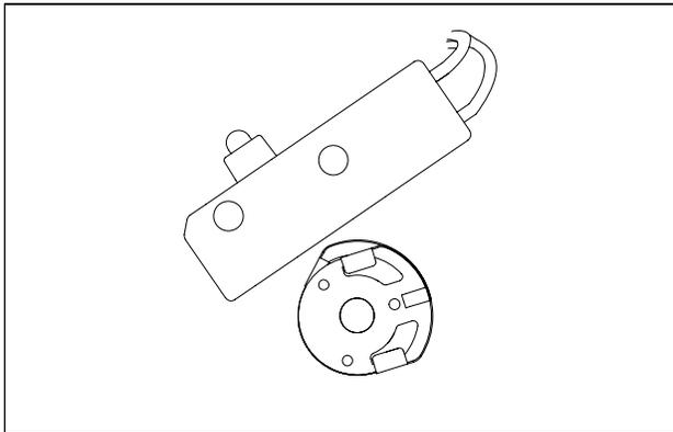
Fig. 7 Cams Set for Normally Closed Sensor Function
