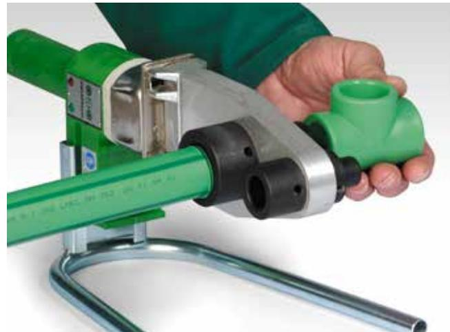
**Warning: Welding heads and heating plate are extremely hot. Always use protective hand and arm coverings to reduce the risk of serious burns.**
