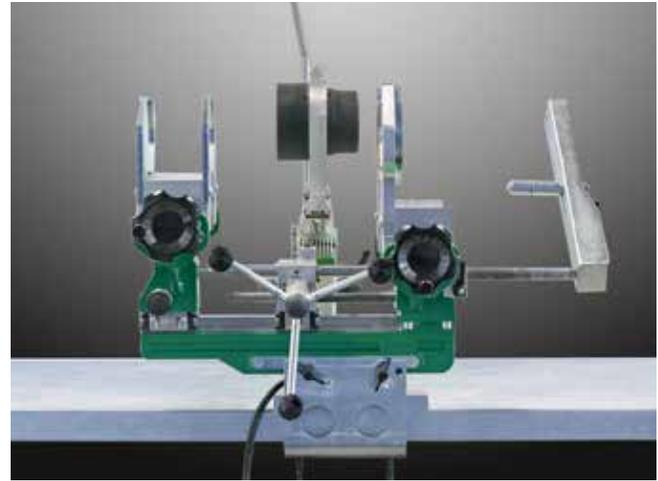
7. Follow the welding time according to the socket fusion welding times table. Lower the welding iron into place and slowly push the fitting and pipe as far as they will go onto the heads.
