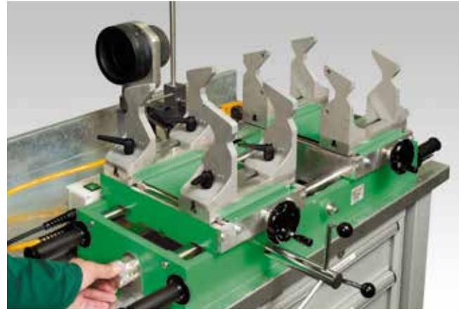
5. Push in the calibration knob and turn the crank as far as it will go. This will slide the pipe to the proper depth.
