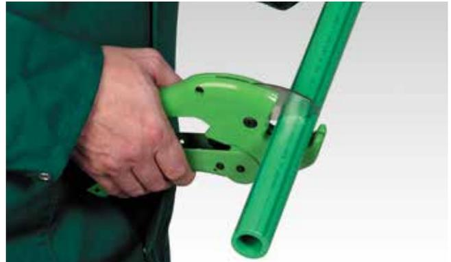
**Always ensure that cutters are sharp. Cutting pipes with dull or damaged ratchet cutters can cause the pipe to crack.**
