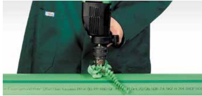
Drilling through the pipe wall.
