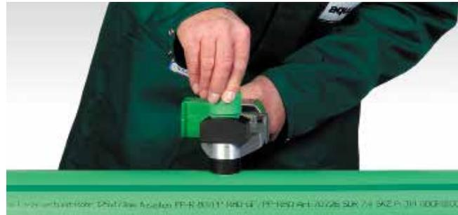
Heating up the pipe and fitting.
