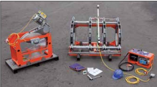
Inspect the welding machine and heating iron.
