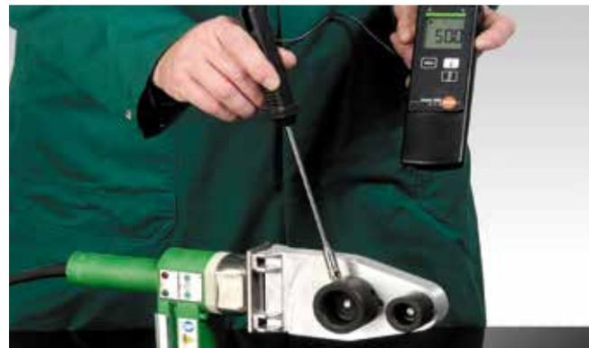
**Important:** If the pipe or the air around it is below 40 °F (5 °C), heating times are increased by 50%. Remember to take greater care with the pipe as it can become brittle in cold temperatures. Using power cutters on cold pipe can cause cracking and is not recommended. Use standard ratchet or wheel cutters instead. Never pre-heat the pipe beyond 100 °F (38 °C).
