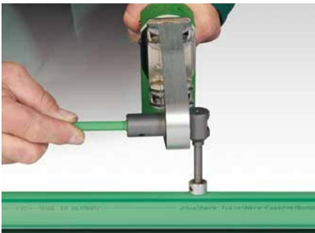
6. Remove the pin from the repair tool and the repair head from the hole. Insert the repair pin into the hole and hold it in place for 15 seconds.
