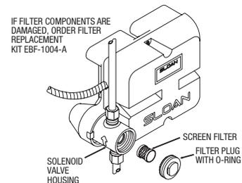
Clean the screen filter using fresh tap water only. If necessary, use a small brush to clean. Use caution while cleaning to prevent damage to the solenoid screen filter. If any filter components are damaged, order Filter Replacement Kit (EBF-1004-A).
