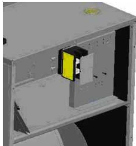
9. Reinstall the access panel removed in Step 2. Ensure the panel edge does not cut into the wire insulation.
