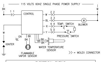
ELECTRICAL RATING 115 VOLTS 60HZ LESS THAN 12 AMPS
