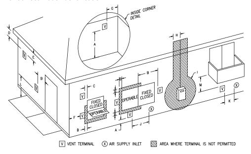
Figure 1 - Vent Terminal Clearances
