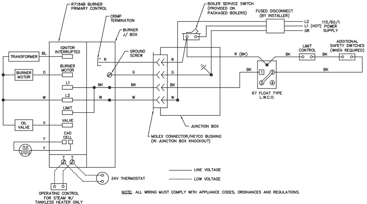
**Figure 4.3: Steam with Float Low Water Cut-Off**
