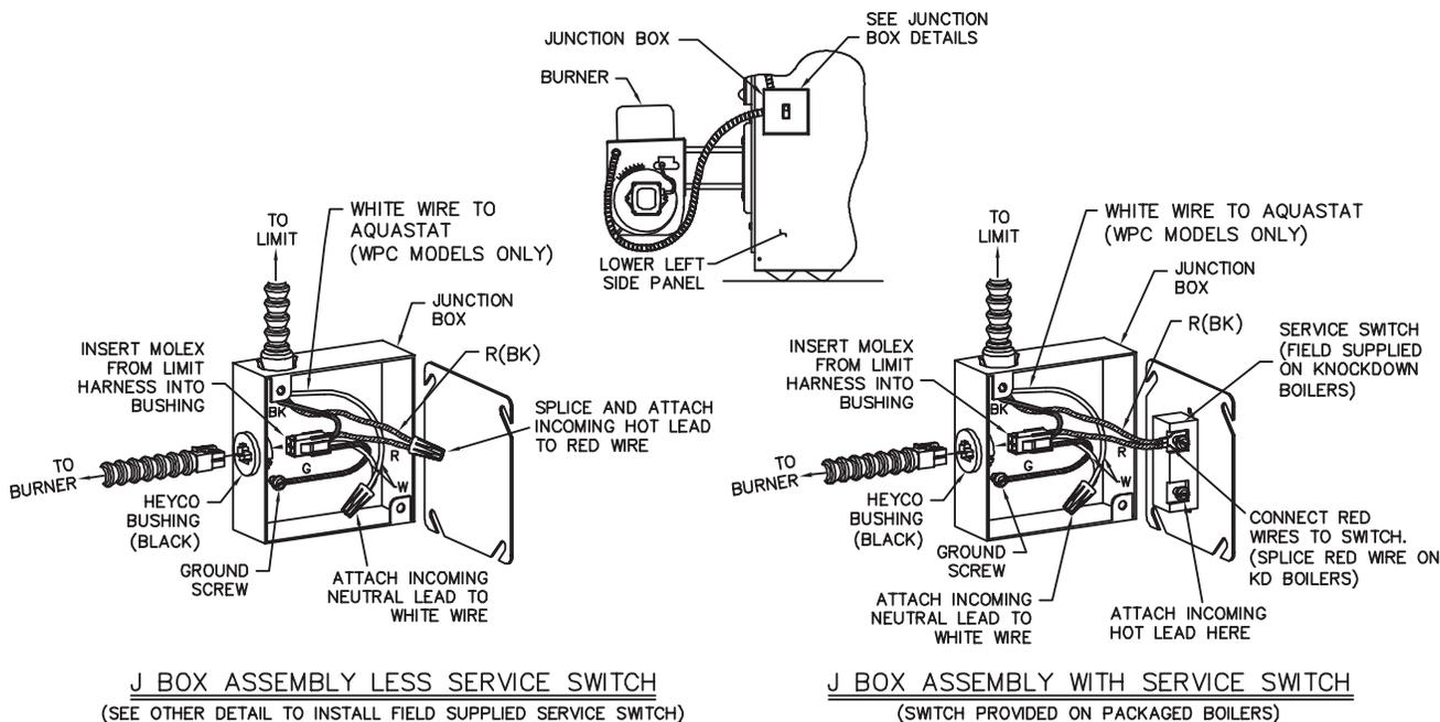
Figure 4.1: Junction Box Wiring
