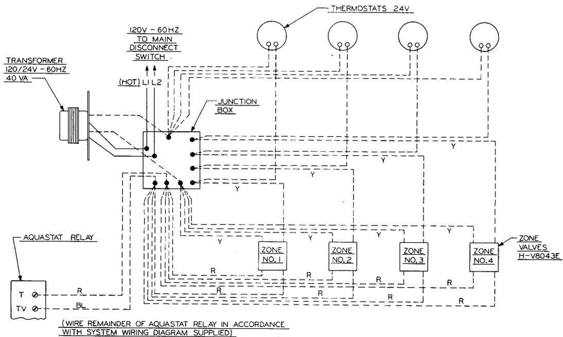
(WIRE REMAINDER OF AQUASTAT RELAY IN ACCORDANCE WITH SYSTEM WIRING DIAGRAM SUPPLIED)
