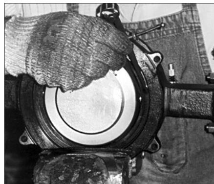
Figure 8 – Shows how to measure the gap between the body seat pocket ID and the disc OD
