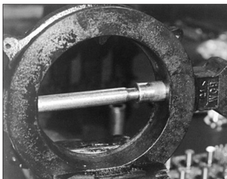
Figure 7 - Shows the stem bushing flush with the flow path surface.
