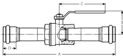
Series 589 Ball Valve is a full port valve with Vic-Press Schedule 10S ends for fast, easy installation. The valve, with Vic-Press Schedule 10S ends, is designed for service to 300 psi/2065 kPa.
