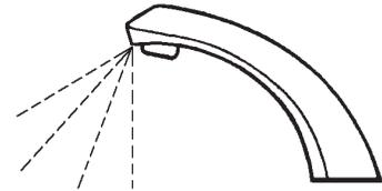
2. As the user's hands enter the beam's effective range (beneath the spray head), the beam is reflected into the receiver "eye" and activates the valve. Tempered water flows from the faucet into the sink until the hands are removed from the sensor's beam or until the faucet reaches the automatic time-out limit setting (factory set at 30 seconds).
