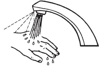
3. When hands are moved away from the OPTIMA faucet, the loss of reflected light initiates an electrical signal that deactivates the valve, shutting off the water flow. The circuit then automatically resets and is ready for the next user.
