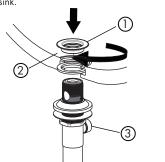
Place one end of spring clip (1) on the end of pivot rod (2) . Insert rod through hole in lift rod strap (3) . Secure with spring clip (1) .
