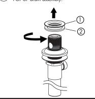
Place the rubber washer (2) to underside of the flange (1). Insert the threaded end of the drain body up through the drain hole and attach flange to the body with the pivot hole (3) pointing to the rear of the sink.
