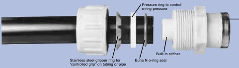
Stainless steel support collar on female pipe thread fittings assures lock-proof connection to metal pipe threads
