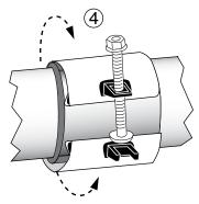
**Note:** If necessary (because of water pressure) Step 4 and Step 5 can be performed beside the pipe break. Slide the clamp over the break after the bolt head has been snapped in place.
