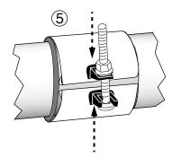
**Step 6** • Tighten all nuts evenly in 10 ft-lb. increments. Keep torques as evenly balanced as possible. Use a wrench with at least a 12" handle.
