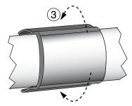
**Step 4** • Back off nuts of shell to the end of the bolt, **DO NOT REMOVE.** Separate clamp and wrap it around the gasket cartridge).
