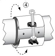
**Note:** If necessary (because of water pressure) Step 4 and Step 5 can be performed beside the pipe break. Slide the clamp over the break after the bolt head has been snapped in place.
