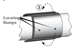
**Step 4** • Back off nuts of shell to the end of the bolt, **DO NOT REMOVE.** Separate clamp and wrap it around the gasket cartridge, positioning it so the locating bumps are between the lugs (in the shell gap).
