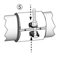
**Step 6** • Tighten all nuts evenly in 10 ft-lb. increments. Keep torques as evenly balanced as possible. Use a wrench with at least a 12" handle.
