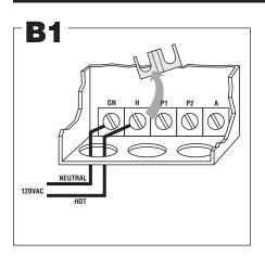
btween H and P1. Connect the hot lead of the input voltage (120 VAC, 60 HZ) to terminal H. Connect the neutral lead to terminal GN. 120 VAC, 60 HZ must be supplied to terminals H and GN for internal operation of the control.
